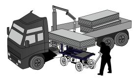
3 Horizontal unloading of stacks of drywall on trestles or vertical unloading of stacks of drywall in ErgoLoader
